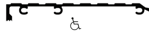
1/2" Tileback aluminum saddle threshold (ADA) available in 4-1/4" and 6-1/4" widths. Inswing use only
