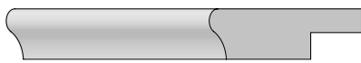
STOOL CAP Serves as the interior extension of the window sill. Immediately below the stool cap a piece of horizontal trim called the apron is applied against the wall (as pictured above).
